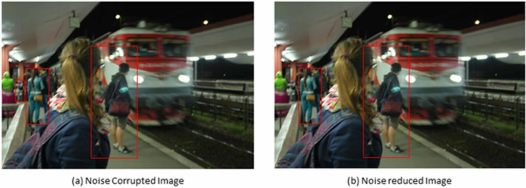
Figure 8. Example of better detection performance after denoising (Before denoising: TP=2, TN=1, FN = 2, FP = 1; After denoising: TP=2, TN=2, FN=2, FP=0).
