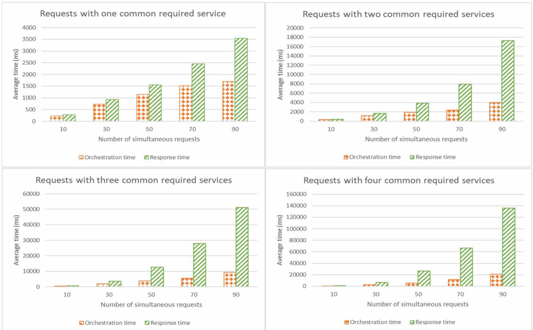
Figure 19. Orchestration time and response time for the optimization case with various input requests
