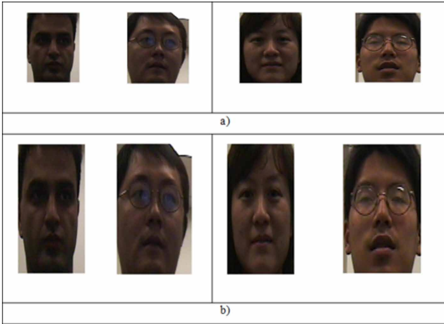
Figure 4. Experimental outputs of the proposed face SR technique: (a) Input video frame; (b) SR output
