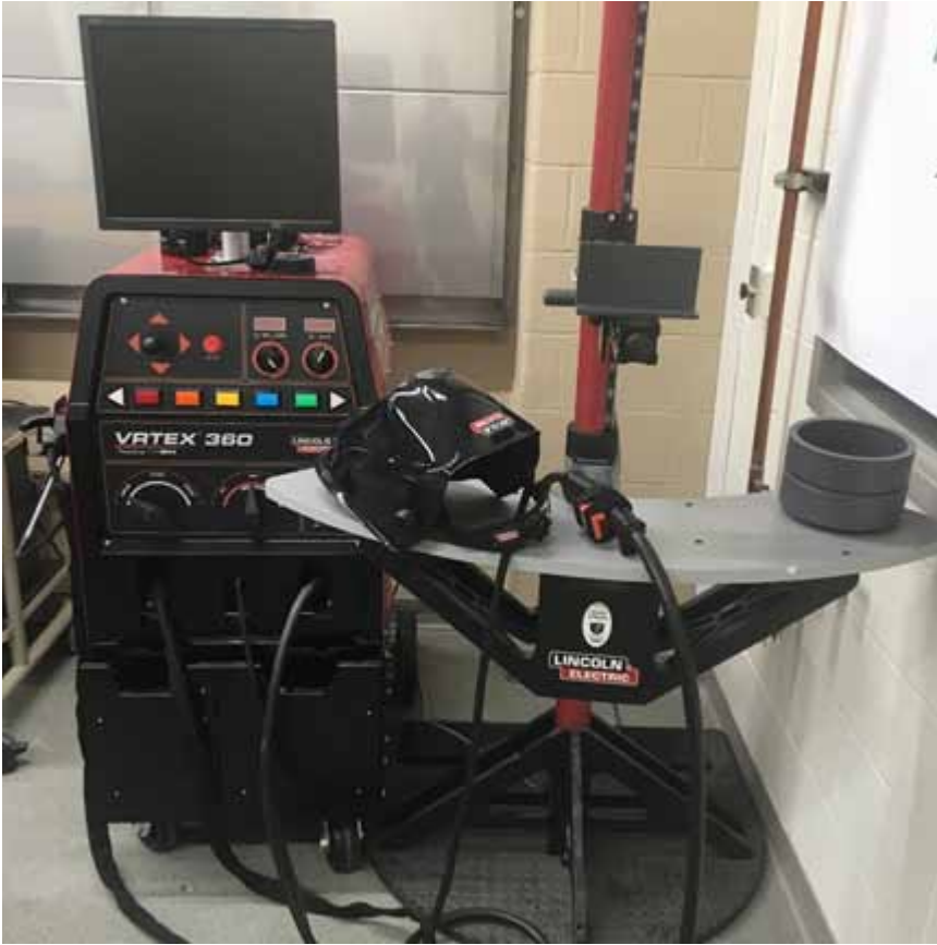
Figure 1. VRTEX 360, LINCOLN welding simulator
