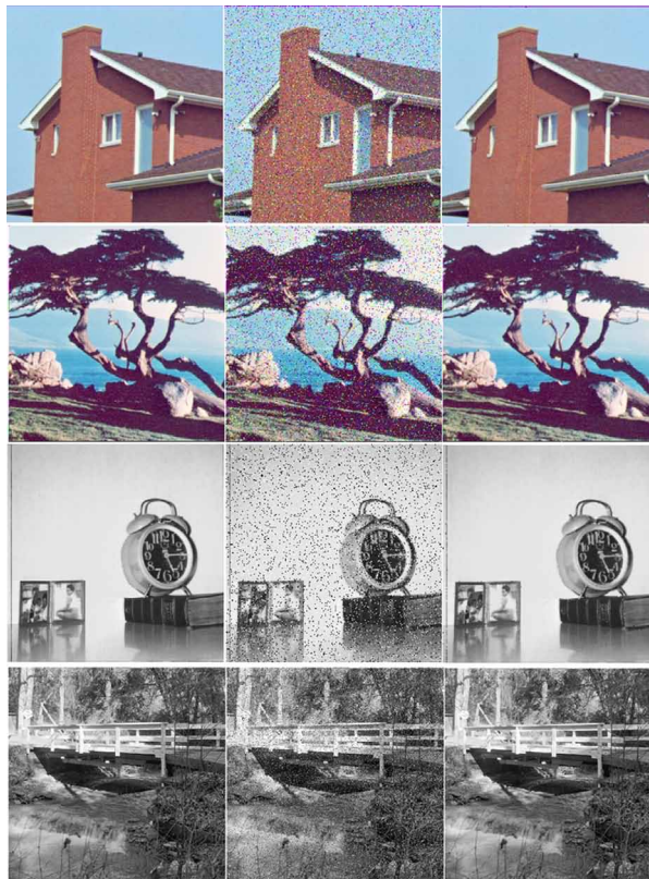
Figure 1. Image denoising examples using conventional approaches. Images on the left are the original images. Middle images have been corrupted by impulse (top) and Gaussian (bottom) noise respectively. Images on the right are the results of filtering by median (top) and Wiener adaptive (bottom) filters respectively.
