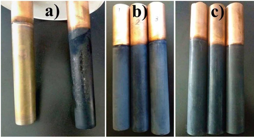
Figure 3. a) Copper tubes with different surface finishing caused by a less or longer anodizing time; b) Blackened surfaces after rinsing with deionized water; and c) Final finishing of black copper tubes. The decrease in the water level caused the difference in height between the pipes of the black section.
