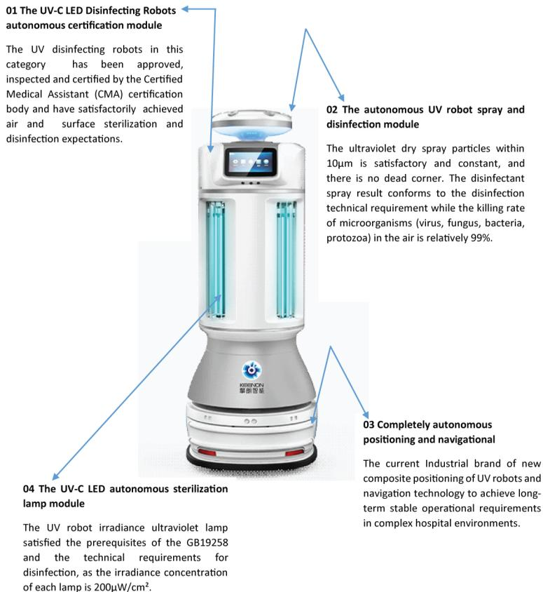
incapacitating microorganisms, like protozoa, viruses and bacteria from replicating (Zheng, Ahmad, & Abbasi, 2020). On this note, the UV-C LED disinfecting robots energy level are very effective, chemical-free and environmentally-friendly in a way to prevent microorganisms from multiplying in any environment especially within the healthcare facilities where the risk of hospital acquired infection are high.
