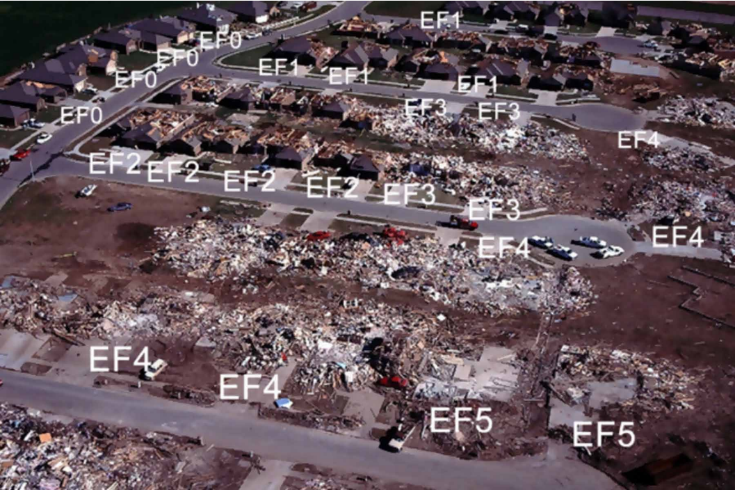
Figure 2. Gradations of damage ranging from EF0 (upper-left corner) to EF5 (lower-right corner) (NOAA, 2019b)
