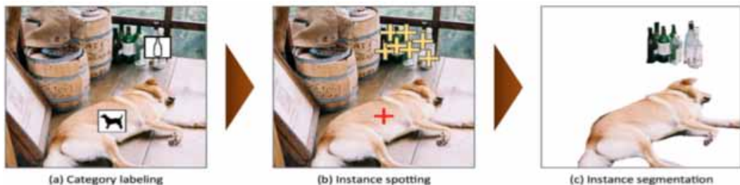
Figure 9. (a) category labeling categories present in the image (b) marking the instances of the labeled categories (c) segmenting each object instance
