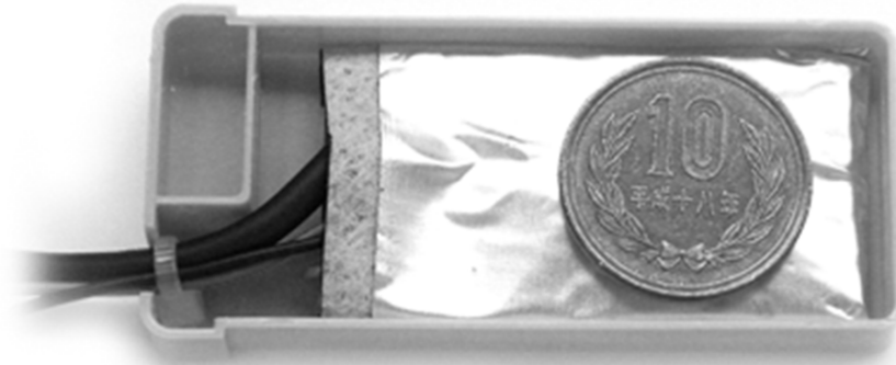
Figure 2. Assembling the Pokéga Type 1. The user places the Pokéga board in the mint candy case and uses a 10-yen coin as a shield against beta radiation.
