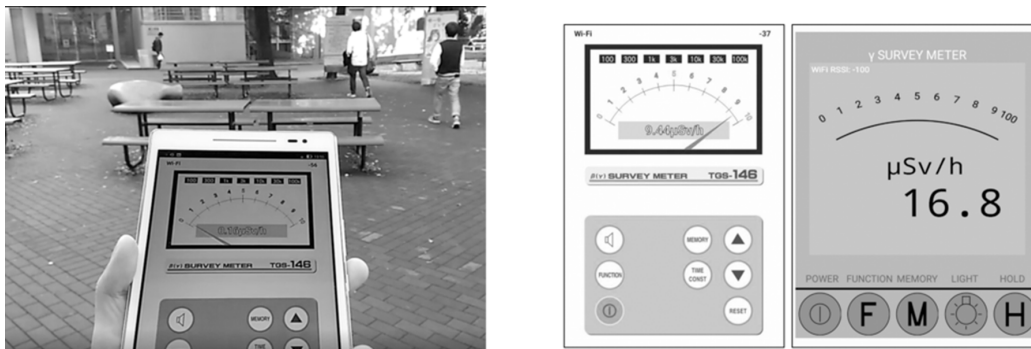
Figure 5. USOTOPE in use: terminal with the application running (left), screen captures of two types of measuring instruments emulated by the application (right)
