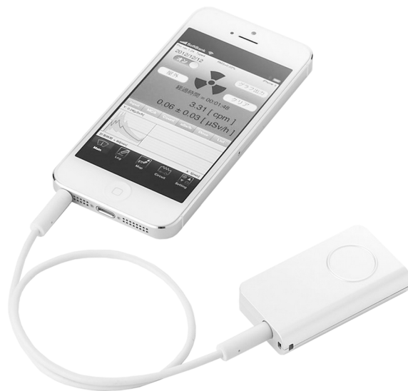
Figure 1. Exterior view of the Pocket Geiger (Pokéga) Type 4. Pocket Geiger is available in models from Type 1 to Type 6.
