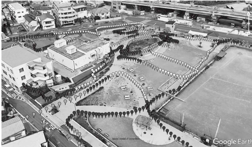
Figure 9. Prototype of GPS-based USOTOPE: assuming that high levels of radioactive material were placed on the campus, radiation levels were visualized based on GPS location
