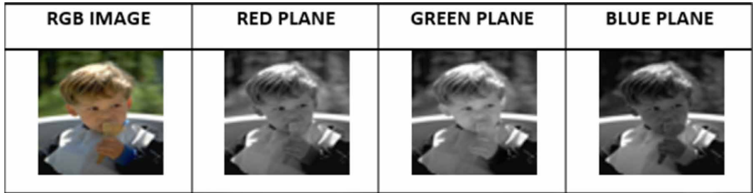
Figure 7. Distribution of an RGB image into red, green and blue color planes
