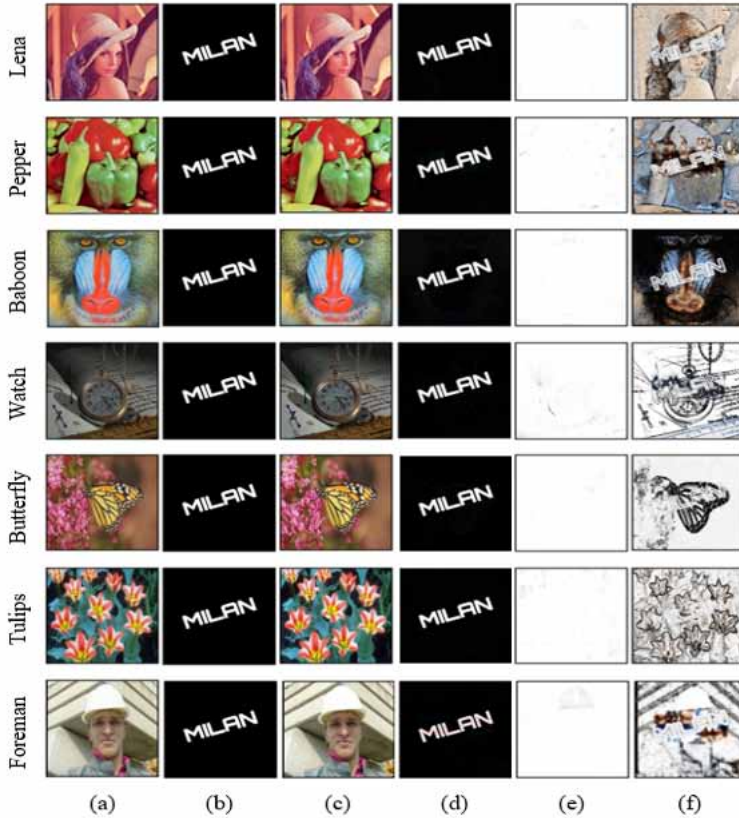
Figure 5. Watermarking images: (a) cover images, (b) watermark images, (c) watermarked images, (d) extracted watermarks, (e) SSIM for cover images/watermarked images, (f) SSIM for extracted watermark
