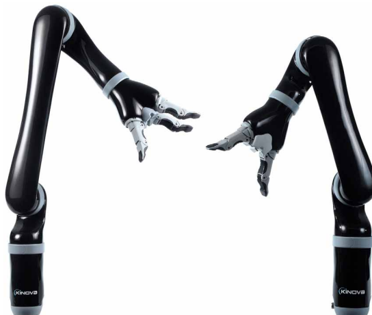
Figure 4. JACO 2 and MICO 2 4 DOF versions side by side. Figure courtesy of Kinova.
