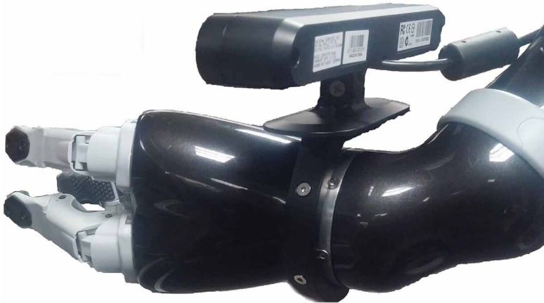
Figure 9. A Microsoft Kinect attached to JACO2 wrist. Figure courtesy of University of Colorado Boulder, Correll Robotics Lab.
