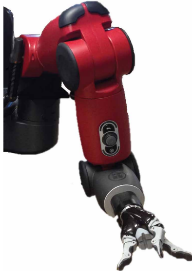
Figure 7. Kinova's gripper KG-3 installed on a Baxter robot. Figure courtesy of Rethink Robotics.
