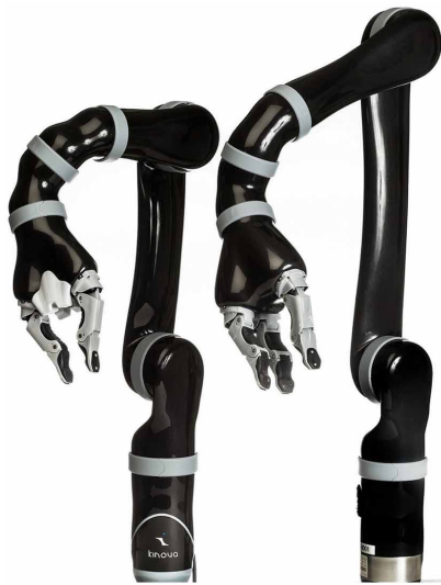
Figure 3. MICO 2 and JACO 2 6DOF versions side by side. Figure courtesy of Kinova.
