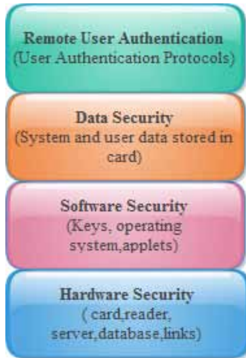
Figure 1. Multi-layer security for smart card-based applications
