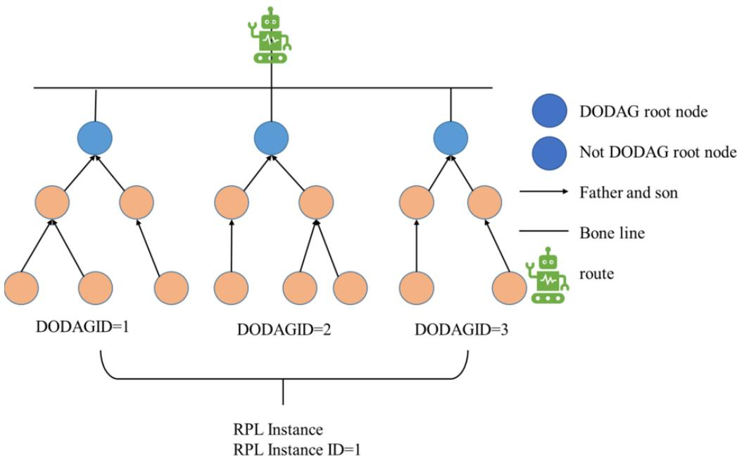
a parent and potentially multiple children, and the root being the destination node. DODAGs allow for efficient and adaptable routing, as nodes can dynamically adjust their relationships in response to changes in network conditions. This makes RPL valuable for IoT applications.
