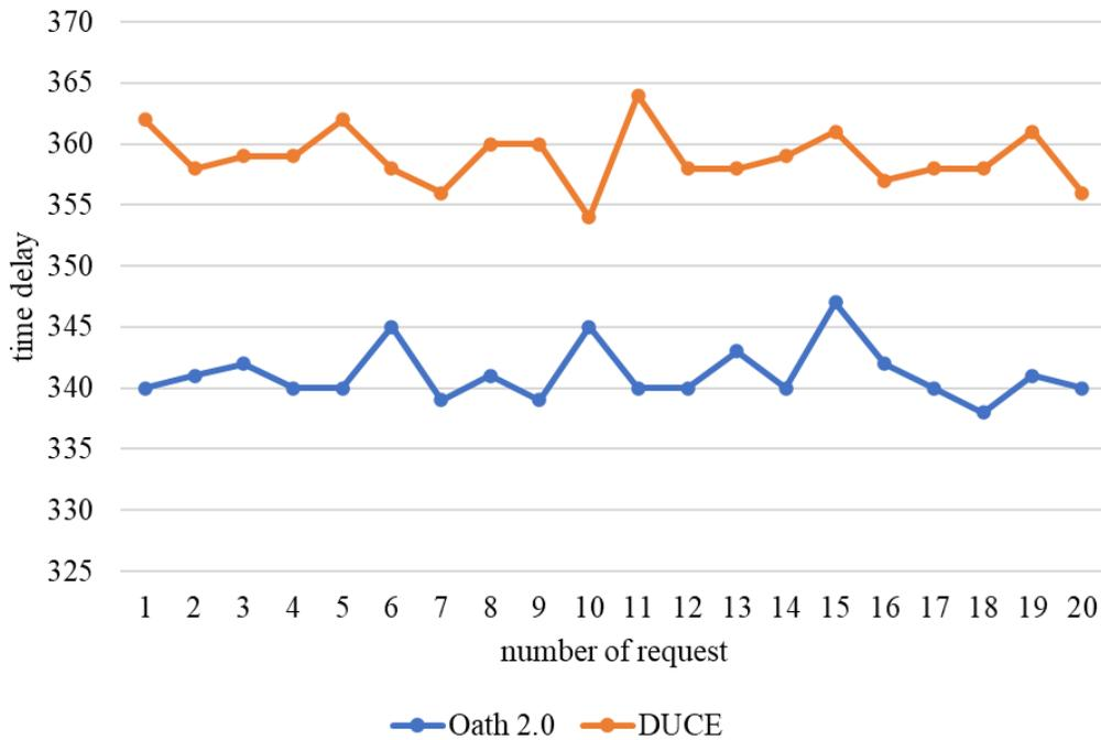
Then, we use JMeter to test the throughput of the authentication, as shown in Figure 9. Figure 9 shows the difference in authentication throughput between the baseline system and DUCE. The graph shows the average result of 20 runs. We found that the peak throughput of our solution was only about 15% lower than that of OAuth 2.0.
