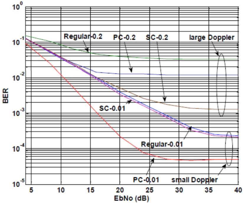
Figure 10. Average BER comparison of the STPC-QPSK and ST-QPSK schemes with the OFDM block size  $N=512$  and the maximum Doppler frequency range from 20 Hz to 100 Hz in TU area
