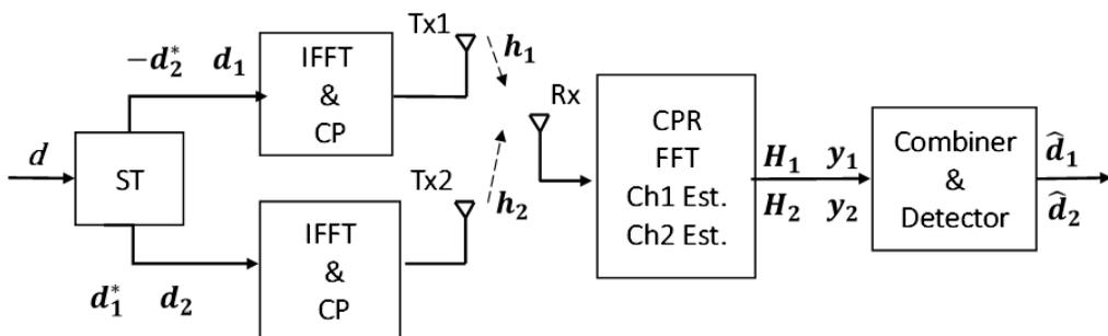
Figure 8. Block diagram of the STPC-OFDM transceiver
