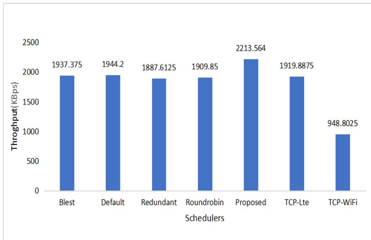
Figure 11. Throughput Comparison in Heterogeneous Networks
