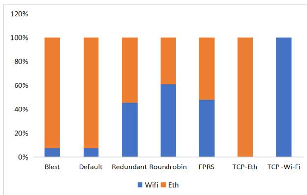
Figure 14. Path Utilization of Schedulers in Wi-Fi-Lte Scenario
