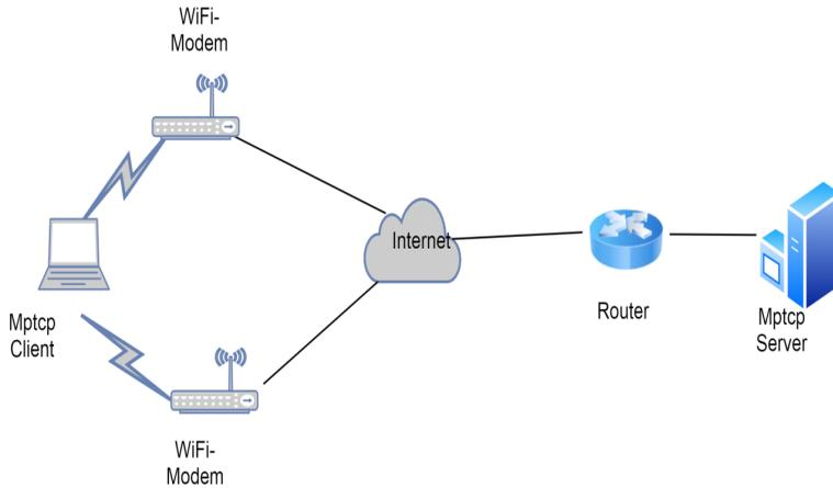
Figure 7. WiFi-Lte Network TestBed
